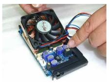
Installing the heatsink/fan onto the processor.
